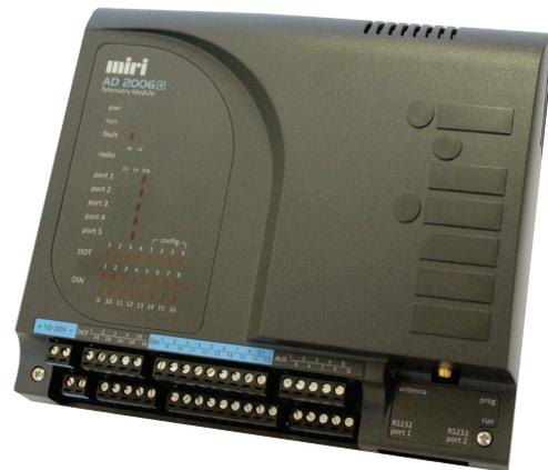
The Miri **AD2006+** Telemetry Module represents an enhanced version of the proven AD2006 series of modules, offering an extremely versatile, digital wireless based product, which finds application in all forms of data acquisition and control systems for industry and public utilities.
